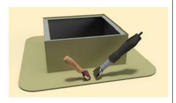
Install roof vent, exhaust fan or pipe cap over curb using recommended screw. See appropriate Vent with Curb Mount Flange installation instructions at roofvents.com for more details.
