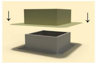
Step 11: Apply a generous amount of heat & pressure to TPO boot to weld it on to the curb & the deck.
